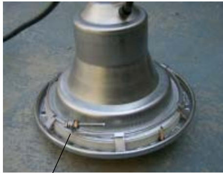
Spring clamp: Remove nut and screw
