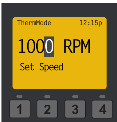
Setting the Thermal Mode Pump Speed
